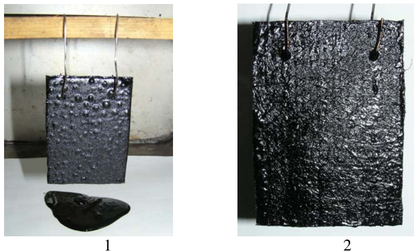
Fig. 2 – View of waterproofing material sample after 30 minutes of its conditioning in oven at 160 °C (1 – upper side, 2 – underside)
